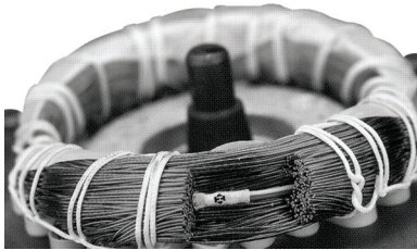
Fig. 44 PTC sensor incorporated in windings
