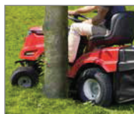
Small turning radius for very good manoeuvrability
