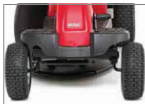
Laterally displaced deck allows mowing close to edges
