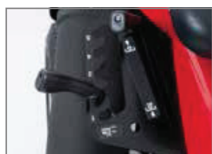
The cutting height can be adjusted between 38 and 95 mm in 5 positions
