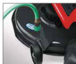
Several lawn tractors by MTD are equipped with a deck wash nozzle for easy cleaning of the deck.
